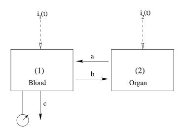
We are interested in the concentrations  $x_i(t)$  of the metabolite in each compartment i. (Note: volumes have been incorporated into the rate numbers, which are *concentration* rates of exchange.) These functions are governed by a differential equation of the form (I'm appending the optional input in parentheses.)
