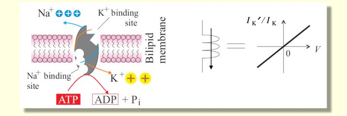
Differential equation (device IV-characteristics) for individual ion pump current
