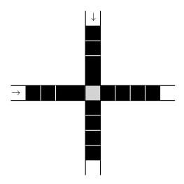
Note that the arrows indicate the intended direction of flow and that the square at the center of the cross is empty. The  $2 \times 1$  pieces of furniture can make it through the crossing only if the  $1 \times 1$  furniture on the other side can flow. Furthermore, the  $2 \times 1$  furniture is stuck in its orientation, unlike the  $1 \times 1$  squares which could flow into the wrong pipe.
